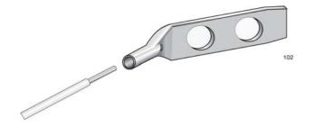
Figure 45. Attaching the Grounding Wire to the Grounding Lug
